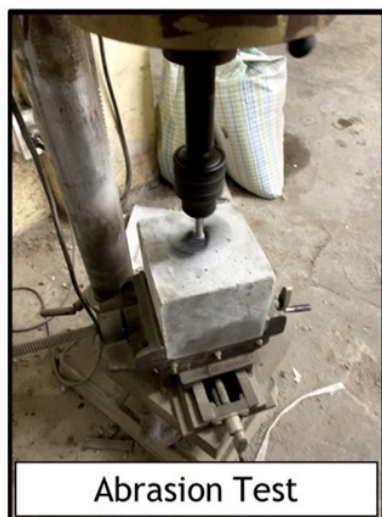
Figure 6 Abrasion test as per ASTM C944
