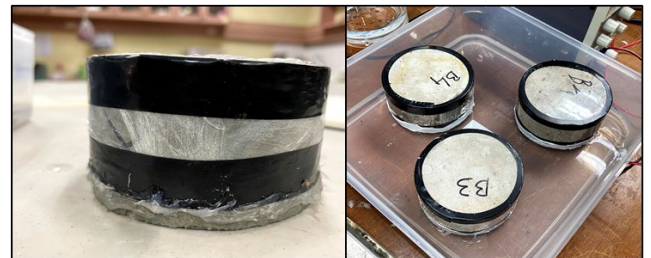
Figure 3 Actual sealed sample used for sorptivity test
