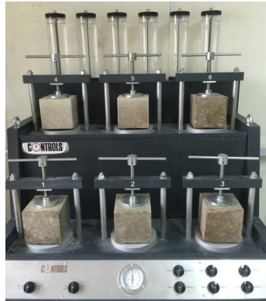
Figure 2 Water permeability setup for testing concrete
