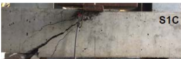
Figure 5 Crack patterns of specimen S1-C (control)
