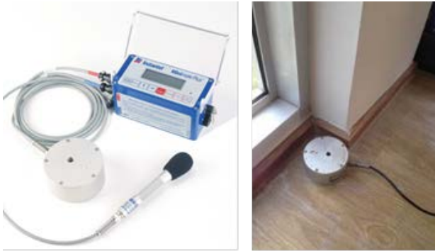
Figure 7 Instrument for PPV measurement at site
