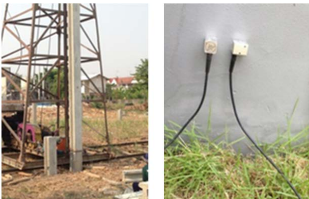
Figure 9 Measurement of the acceleration at site
