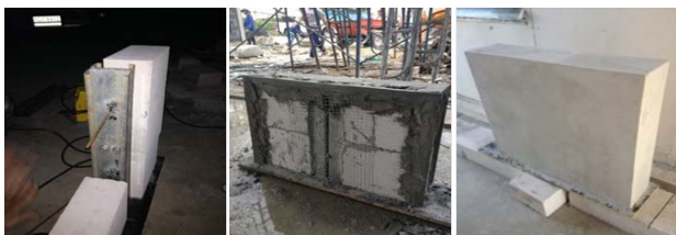
Figure 4 Production of the experiment samples
