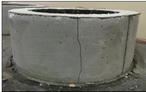
Figure 2 Typical cracking of control mortar
