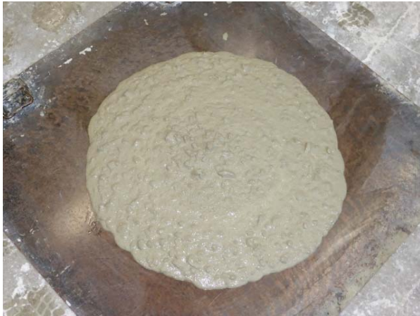
Figure 12 Slump flow of air-SCC
