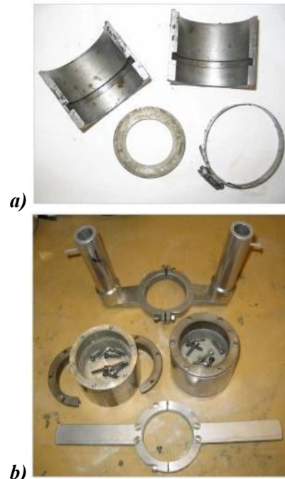
Figure 5 a) casting molds (metal casing and rings) and b) testing apparatus
