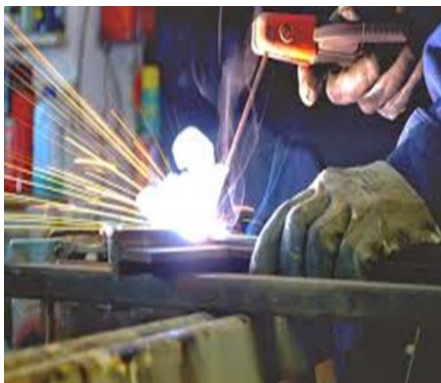
Figure 6 Welding of the structure of a wood lathe
