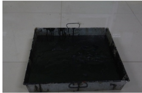
Figure 1 Asphalt cement AC 60/70
