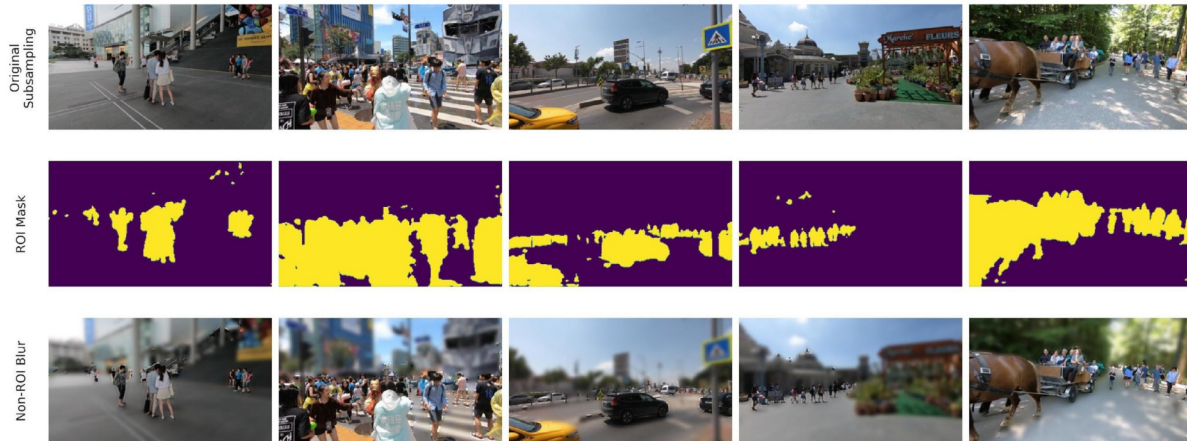
Fig.3: Examples of preprocessing steps used in this study. Each column corresponds to a different video sequence with a randomly sampled frame. The first row shows the original subsampled frames, the second row shows the binary ROI masks generated by PIDNet, and the third row shows the preprocessed frames after applying non-ROI blurring.
