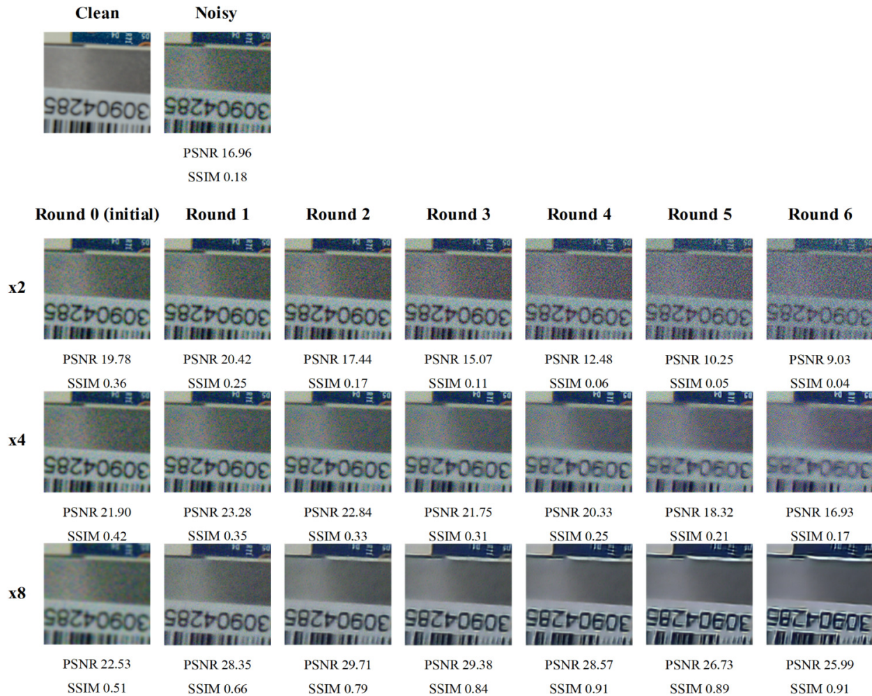
Fig. 8: Sample output of NLR2NSR framework for NIND dataset with x2, x4, and x8 downsampling.
