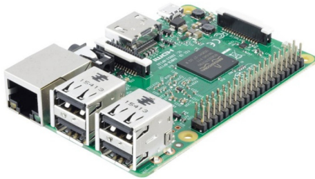
Fig.7: The Raspberry Pi 3B+.
