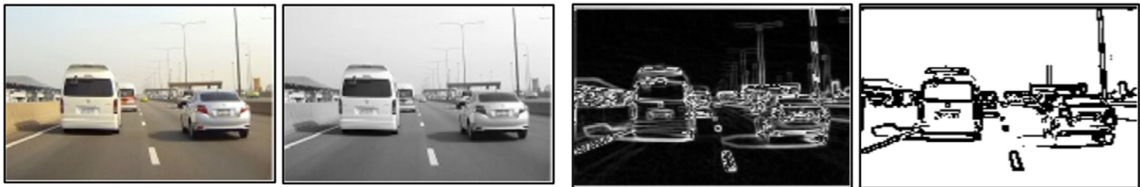
(d) Images of Original, Grayscale, Gradient after Sobel filter and Edge detection.
