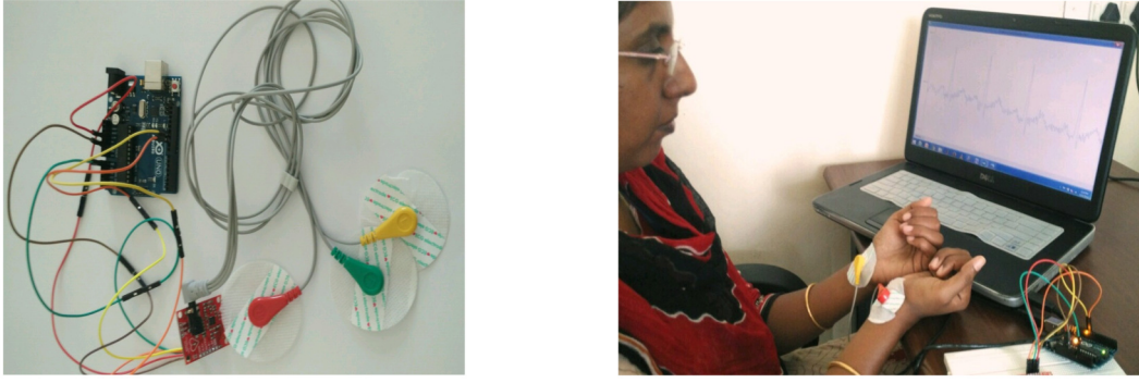
Fig.4: The ECG signal acquired with the test setup (a)The data acquisition system (b)The ECG signal acquired with the test setup.
