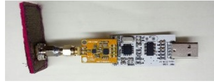
Fig.17: Wearable textile PIFA with a NRF24L01 and a driver board for wireless link evaluation.
