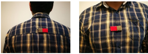
Fig.16: Placement of the antenna in front and the backside of the human body.
