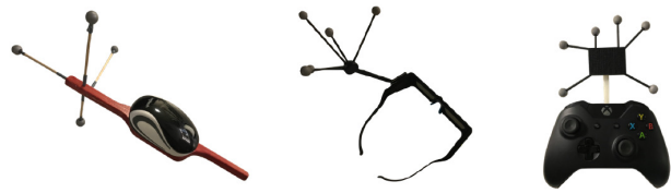
Fig.9: The interactor design for the CAVE interaction system.
