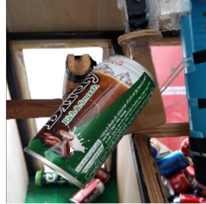
Fig.14: Result of a successful can classification using barcode.
