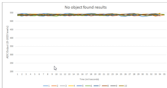
Fig.18: Data from sensor when no object was found.
