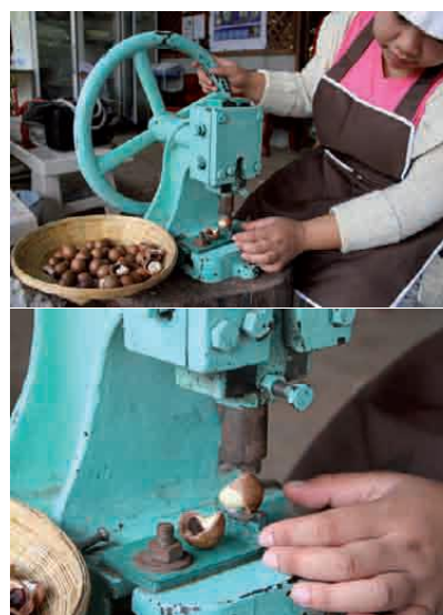
Figure 1 Macadamia nut cracking using the CAERC manual impact system, taken from Krissanasrani (2017) [5]
