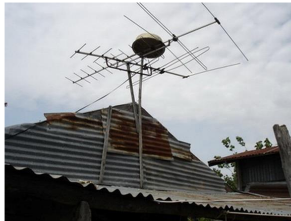
Figure 3 An antenna with a tin basin on the top [12]
