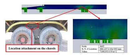
Figure 8 Sensor attachment location on the chassis
