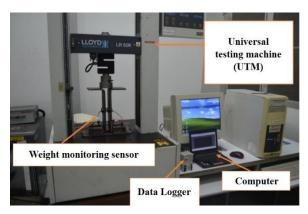
Figure 6 Schematic of calibration equipment
