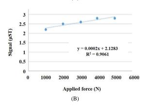
**Figure 10** The linear relationship between the applied force and deflection (A), and the linear relationship between the signal from the sensors and the applied force (B)
