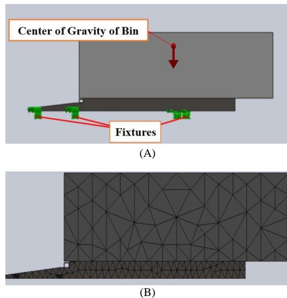
**Figure 3** Boundary condition (A) and element construction (B)
