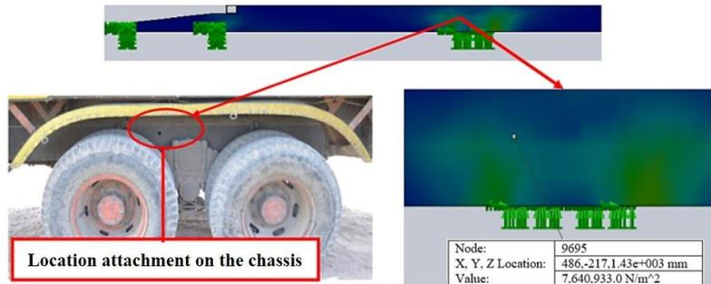
Figure 8 Sensor attachment location on the chassis
