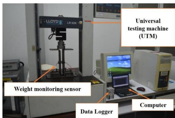
**Figure 6** Schematic of calibration equipment
