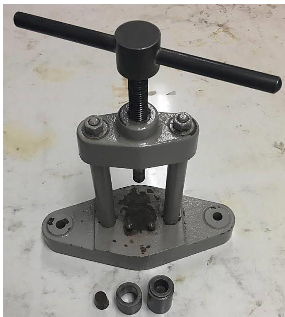
Figure 1 Pelletizing machine used to produce biomass pellets from dry hydrolyzed Napier grass waste
