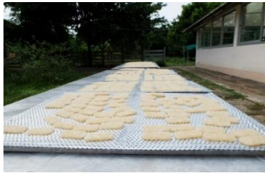
Figure 1 Direct solar drying on a tray
