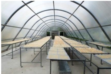
Figure 2 Indirect solar drying with greenhouse dome
