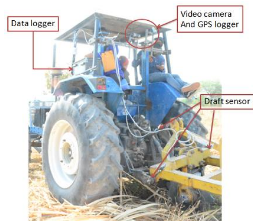
Figure 1 The test was conducted using a Ford tractor, brand model 7840
