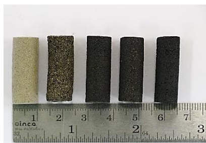
Figure 1 Pellet fuels of lignite and rubber wood sawdust mixture with binders – starch by 10 % wt. (0, 25, 50, 75, and 100% lignite blends)
