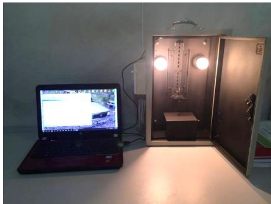
Figure 3 Digital image processing box chamber of this study
