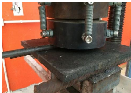
Figure 3 Test of bending strength and elasticity modulus of cement boards
