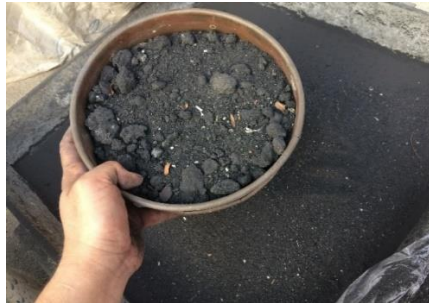
Figure 1 Sieving of coconut shell ash through sieve no.8 for size selection
