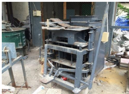
Figure 2 Vibrate compression machine is used to cast the cement boards
