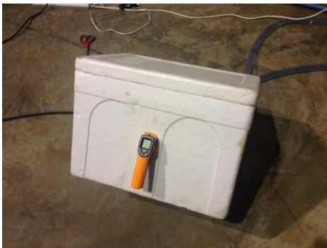
Figure 3 The apparatus set with an infrared gun pointing inside to measure the ambient temperature
