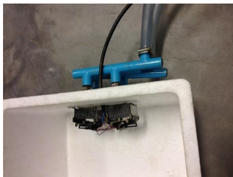
Figure 2 The thermoelectric module inserted through a foam box with top removed
