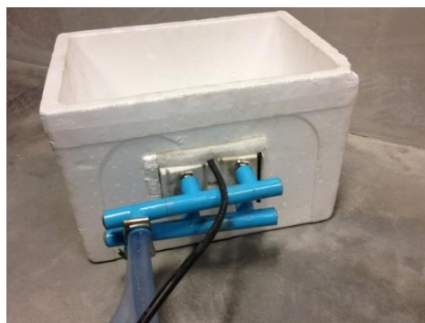
Figure 3 Thermoelectric module with water cooling system shown
