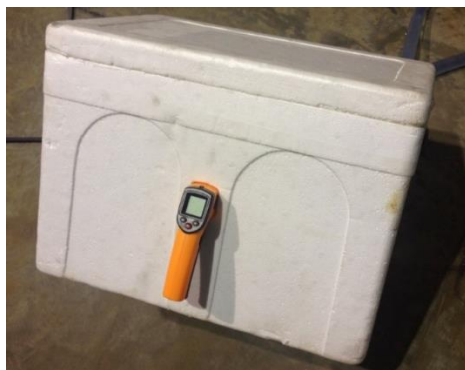
Figure 2 Foam box for data collection with infrared gun installed for temperature measurements within the space
