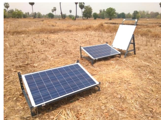
Figure 1 The experiment set up for solar cell with and without mirror
