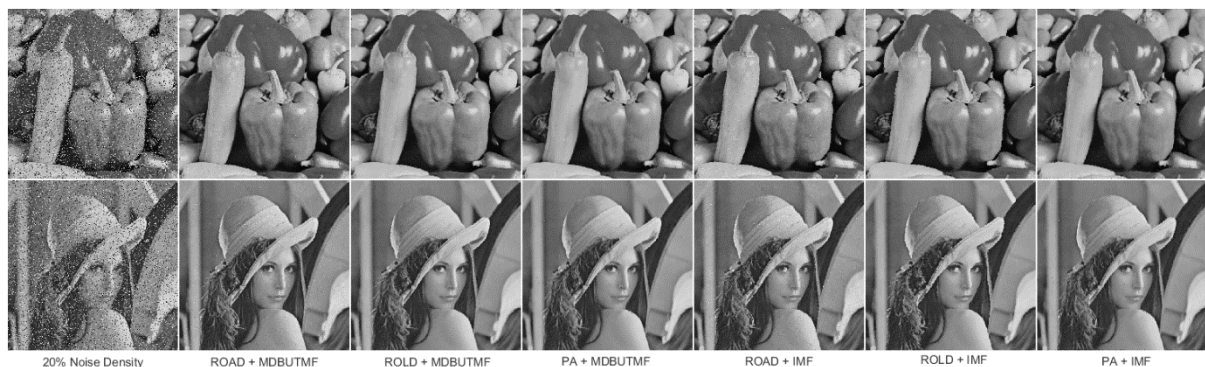
Figure 1 The Results of the proposed algorithm and various algorithms for ‘Lenna.jpg’ and ‘Peppers.jpg’ grayscale images corrupted with 20% noise density
