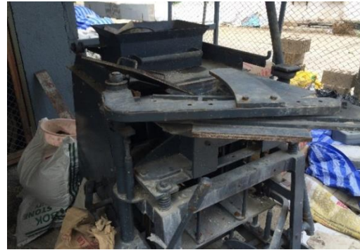
Figure 5 Vibratory compression machine is used to cast the cement boards
