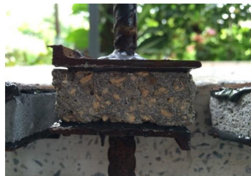
Figure 6 Sample for tensile strength perpendicular with surface test
