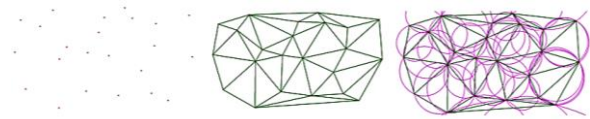
Figure 1 Left is scattered points, the center is Delaunay triangulate and right is circumcircle.
