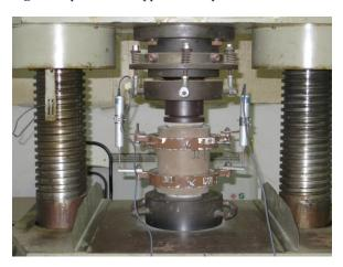
Figure 6 Jacketed concrete cylinders under compression testing
