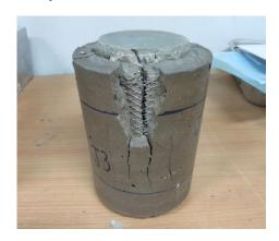
Figure 8 Tearing of the expanded metal mesh
