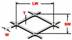
Figure 3 Non-galvanized expanded metal mesh
