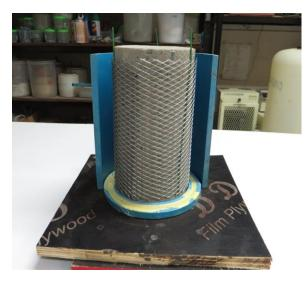
Figure 5 Specimens wrapped with expanded metal mesh
