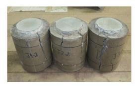
Figure 9 Failed J1, J2 and J3 specimens (left to right)
