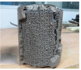
Figure 2 Expansion and formation of gas bubbles of geopolymer mortar when galvanized wire mesh was used
