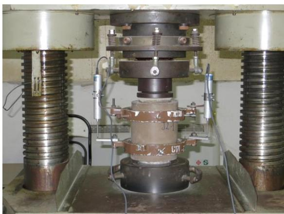
**Figure 6** Jacketed concrete cylinders under compression testing
