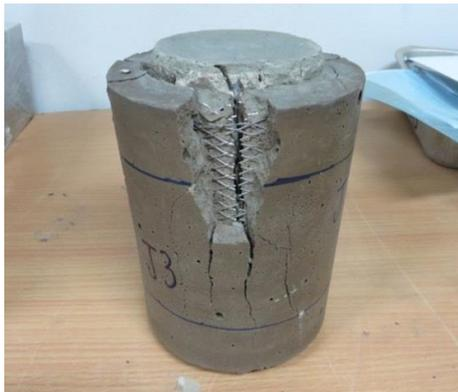
**Figure 8** Tearing of the expanded metal mesh
