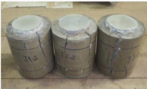
**Figure 9** Failed J1, J2 and J3 specimens (left to right)
