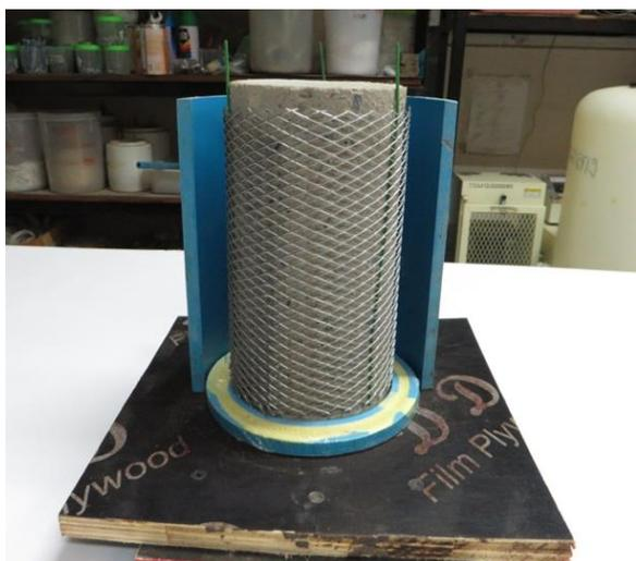
**Figure 5** Specimens wrapped with expanded metal mesh
