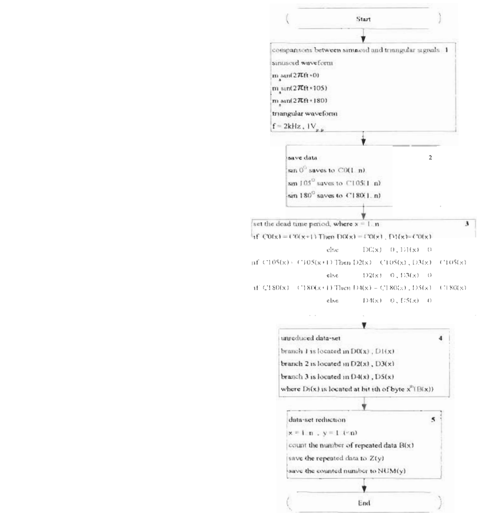
Figure 5: Procedures of Pulse Width Calculations and Data Compression
