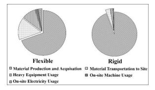
Figure 3 Pie charts showing GHG emissions in each construction process
