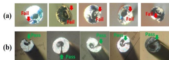
Figure 8 Wire cut characteristic under micro scope (30X) compare (a) before and (b) after machine adjustment
