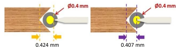
Figure 7 The distance of blade and wire groove slot (a) before and (b) after adjustment
