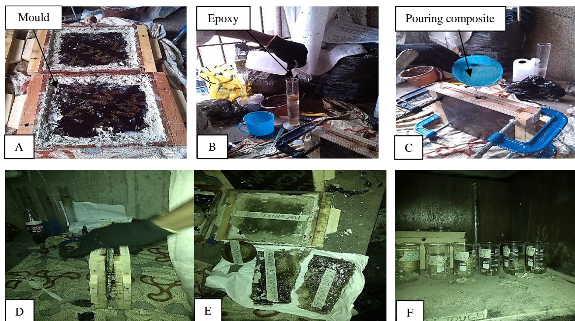
Figure 1 A - Preparation of the mould for casting; B – Measuring epoxy in a cylinder before mixing with orange peel particles; C – Pouring mixed epoxy and orange peel particulate into a prepared mould; D – Dismantling the cured epoxy composite after 24 hours; E – Solidified epoxy composites; F – OPP-epoxy composite in water
