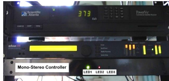
Figure 3 The mono-stereo controller with 3 LEDs indicator
