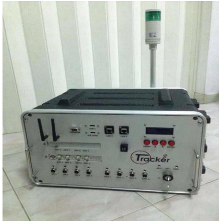
Figure 7 An RFID Controller and RFID Antenna
