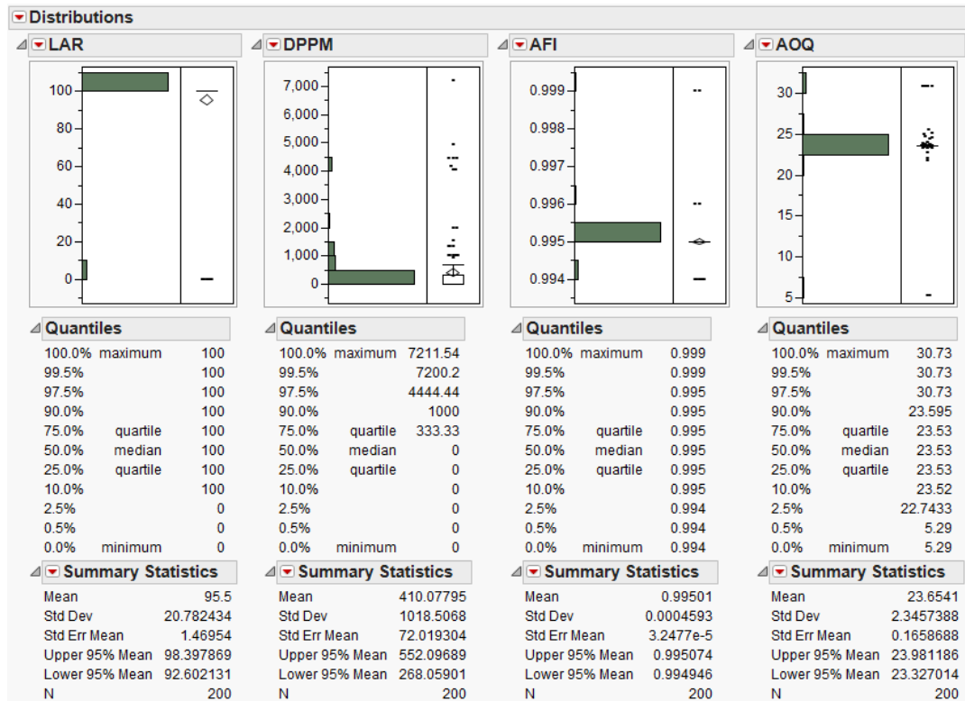
Figure 4 LAR, DPPM, AOQ and AFI result from using CSP-100 sampling plan in 200 lots
