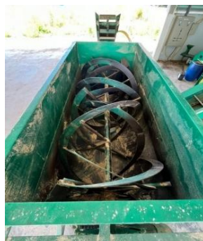
Figure 9 Double helical ribbon blade (1.14 m diameter, 0.51 m pitch).
