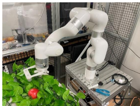
Figure 11 Intel RealSense D435 depth camera of the tomato harvesting robot attached to a UFACTORY xArm 7 robot manipulator
