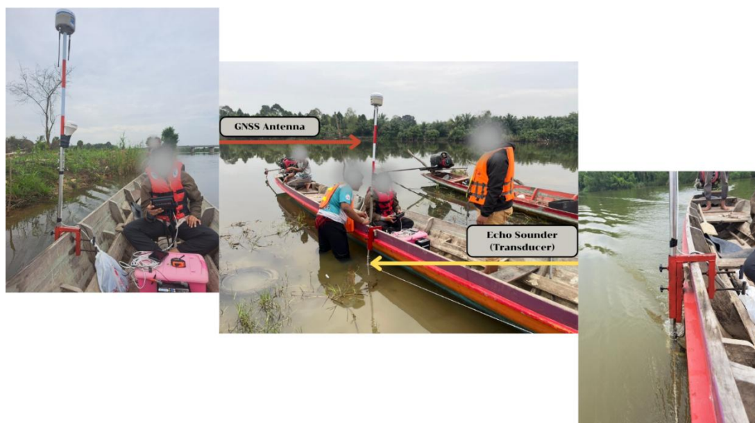
Figure 3 Field setup of the recreational-grade single-beam echosounder (Garmin GPSMAP 585 Plus) integrated with multi-constellation GNSS receiver for accuracy validation at the Songkhla Lake site.
