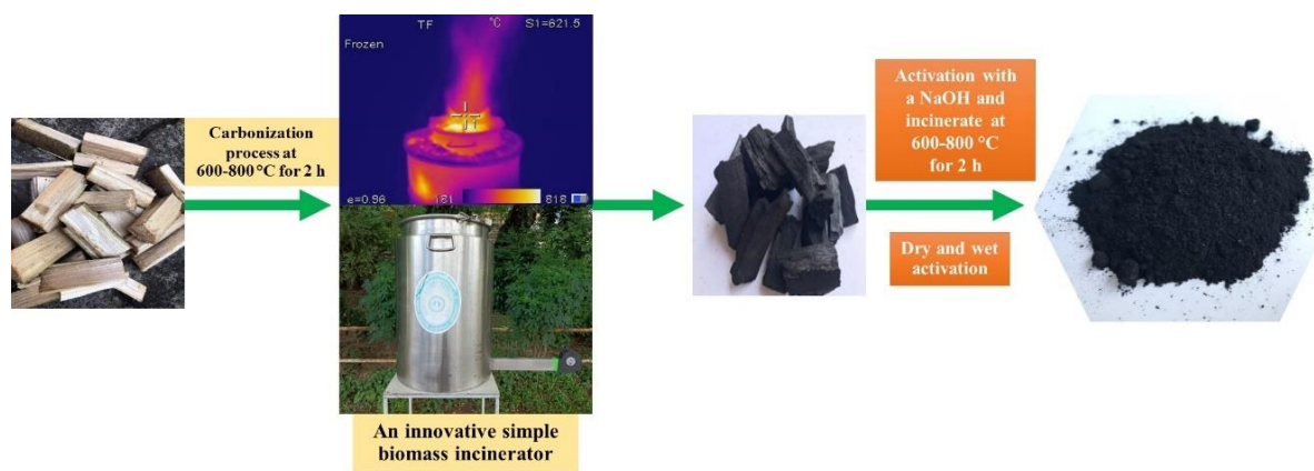
Figure 3 The process diagram illustrates the preparation of carbonized carbon and activated carbon from agricultural waste materials derived from rubber tree branches.
