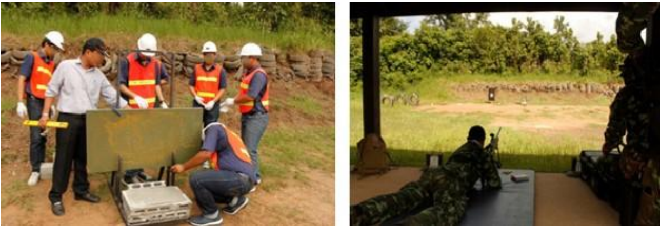
Figure 11 Field test for bullet resistance of HS450-3/AC25/ SS400-6 composite panel.
