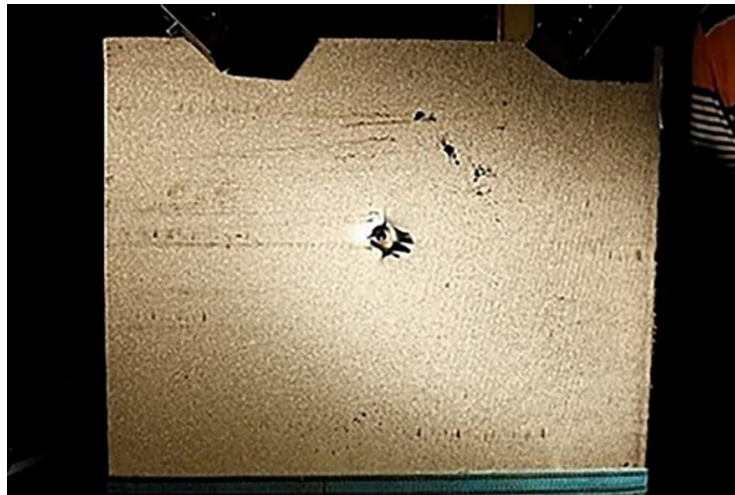
Figure 4 Tested sample after 1 shot penetration.
