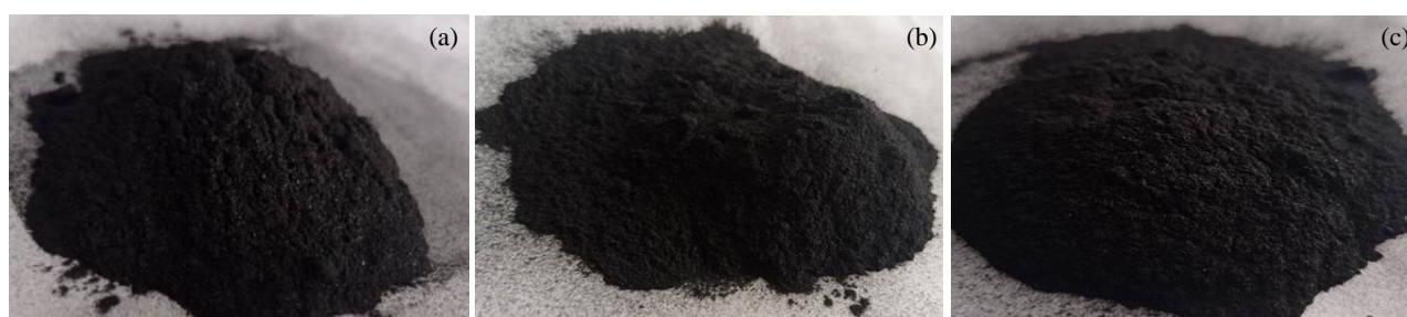
Figure 4 Biochar produced from rubber seed shells at three different carbonisation temperatures: (a) PRC850, (b) PRC900, and (c) PRC 950 (Note: The image of CGA was shown in Figure 3, as it was not included in the biochar production process.)
