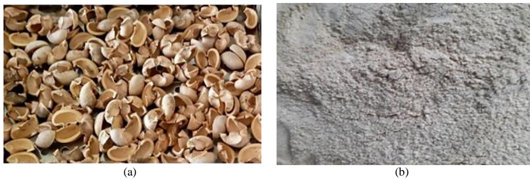
Figure 1 Samples of rubber seed shells (a) dried rubber seed shells (b) ground rubber seed shell
