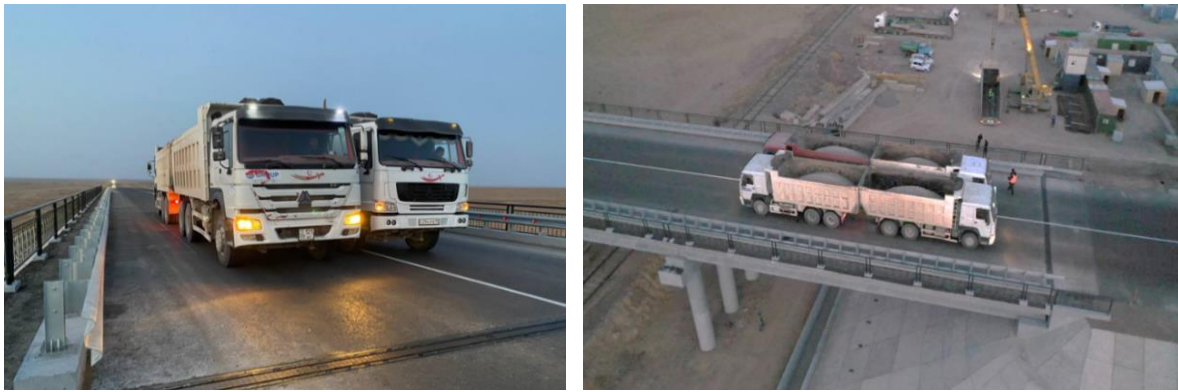
Figure 7 View of the bridge roadway with test loads in the form of loaded vehicles (the first loading scheme).
